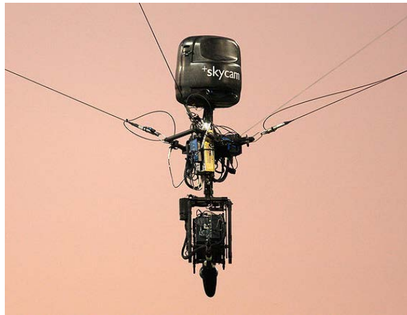
Figure 4 Skycam: a commercialized suspended cable robot
